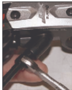
2. Squeeze the lever a few times to extract the pistons. Do not let the pistons come completely out of the cali-
