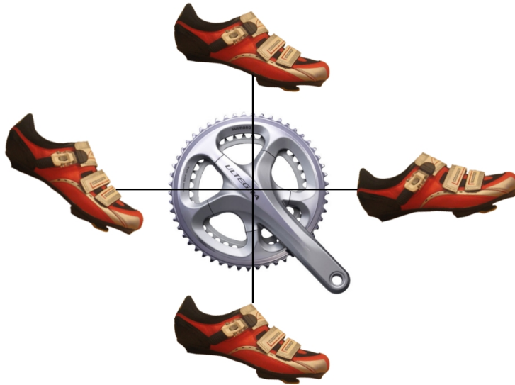
FIGURE 4.4. Picture showing how the pitch angle of the shoe change during one revolution.
