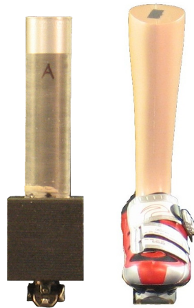
FIGURE 3.1. Picture showing the cylinder mounted to the club foot and the plastic leg in the racer shoe.
